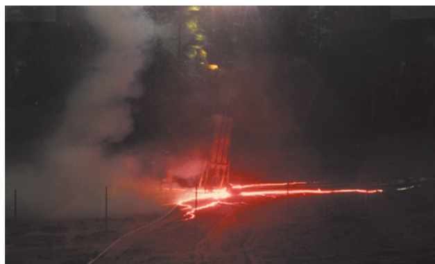
Fig. 13. Photograph of surface arcing associated with the second stroke (current peak of 30 kA) of flash 9312 triggered at Fort McClellan, Alabama. Lightning channel is outside the field of view. One of the surface arcs approached the right edge of the photograph, a distance of 10 m from the rocket launcher [15]
